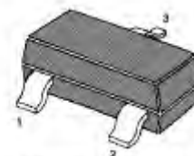
Marking Code: A7 SOT-23 Plastic Package
